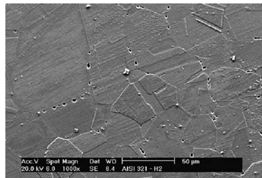
Fig. 11 Sample stabilized at 975 °C and aged at 600 °C for 100 h. Electrolytic etch in oxalic acid solution
